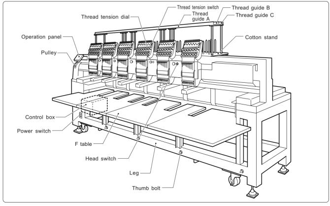
The machine heads are numbered 1 to 6 from the right front.
