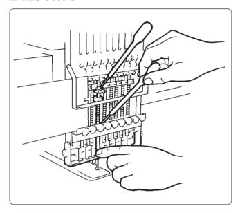
■ Supply oil to the needle bars (18 positions) once a day as shown on the left.
