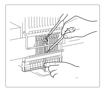
■ Supply oil to the needle bars (24 positions) once a day as shown on the left.
