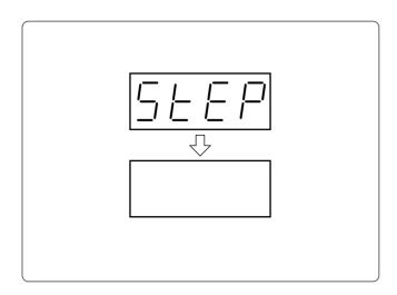
7. After timing adjustment the is finished for each head, set the pulley to the stop position (at 100° of the scale) and press the STOP switch. "STEP" disappears from the display, and the machine enters the standby state.
