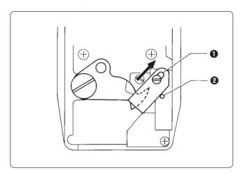
Attach the fixed knife **1** to the pin **2** and move it backward to the end of the slot, then mount it there.
