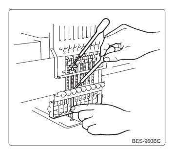
Before operating the machine for the first time after unpacking or after leaving the machine without operation for a long period of time, supply one or two drops of oil to two sections of the needle bar. (See the left figure.)
