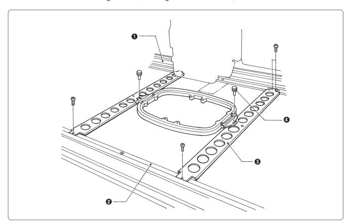
3. When the mounting pitch of the holder base is 550 mm, mount the holder base vertically to the X-axis feed frame 1 and holder base frame C 2 using the thumb bolts 4.
