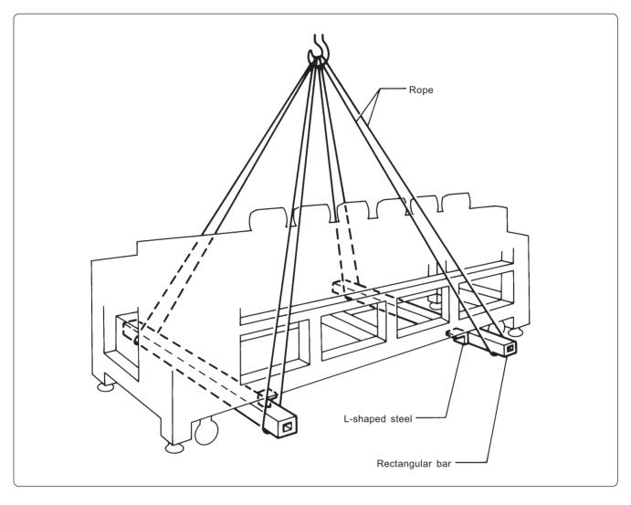
Place two rectangular bars on the four L-shaped steels on the bottom of the machine steel frame. Loop four ropes around the bars and lift the machine.
