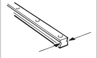
4. Grease the X-feed linear guides (3 positions), the Y-feed linear guides (one each on the right and left), and the linear guide inside the No. 3 bed. Slide the guide to spread grease entirely.
