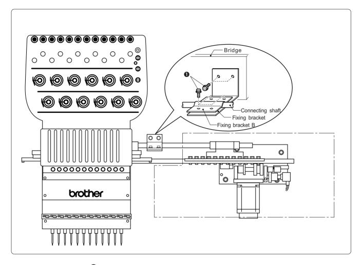
Remove the bolts **1** ,and then detach the fixing bracket B for transportation from the bridge and the connecting shaft.
