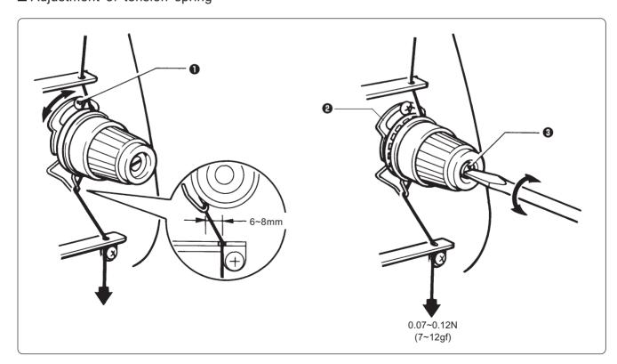
1. The tension spring should be adjusted to 6~8 mm in height and 0.07~0.12 N (7~12 gf) in force.
