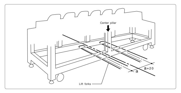
Open the forks of the lift approximately 10 cm to the right from the even position to the center pillar viewed from the rear of the machine, and pass them under the legs to lift the machine.
