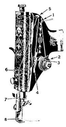
FIG. 11. THREADING THE NEEDLE
