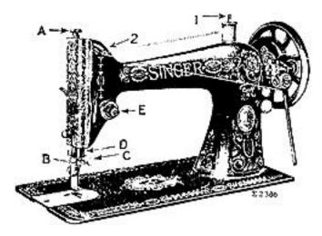
FIG. 5. MACHINE THREADED FOR WINDING THE BOBBIN
