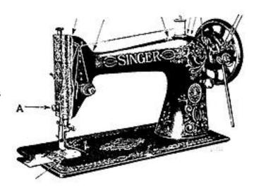
FIG. 17. FRONT VIEW, SHOWING OILING POINTS
