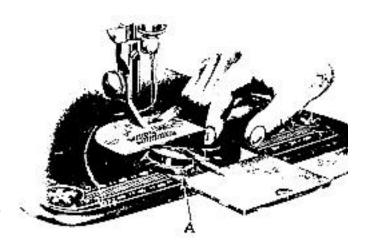
FIG. 4. REMOVING THE BOBBIN
