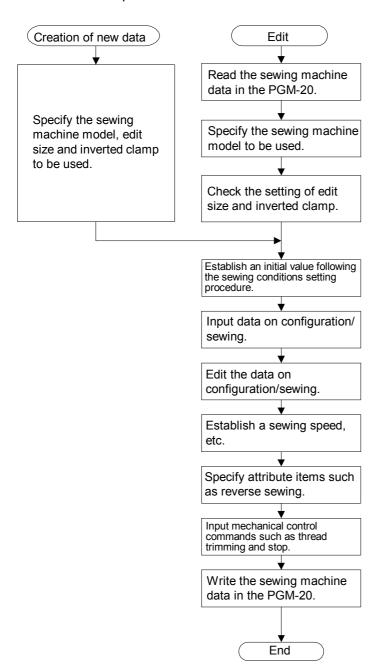
The sewing machine model specified will determine resolution and output data format.
