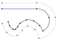
In the case where a compound pattern is used for offset or multi-sewing, an offset compound pattern is created by finding intersection points of the offset component configurations. In the event that graphic intersection points cannot be found, the offset component configurations will be joined by a line. In this case, the offset compound pattern can be deformed.
