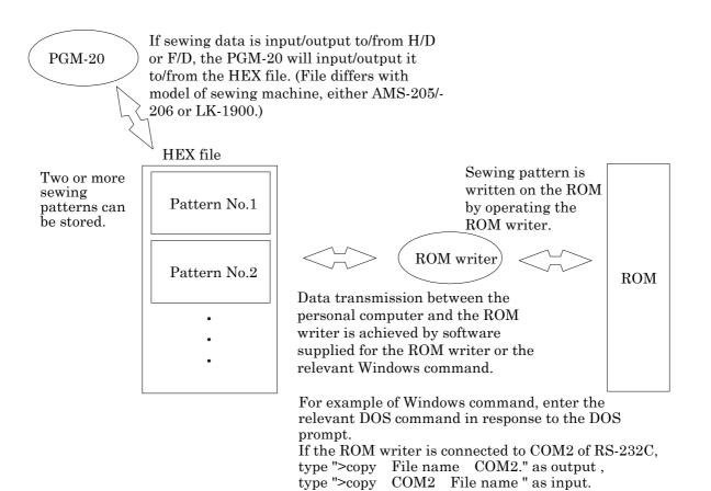
When "H/D read," "H/D write," "F/D read," or "F/D write" prepared in the "Sewing data" contained in the menu bar is executed, reading/writing to/from the HEX file will be performed. At this time, the file is fixed in accordance with model of sewing machine as shown below.
