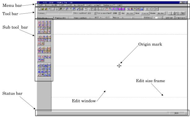
Position the pointer in the function contained in the menu bar, tool bar and sub tool bar to be executed and click the mouse button. Then, operate the personal computer according to the messages given in the status bar or dialog box.
